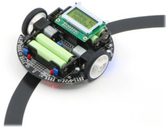
Pololu 3pi robot on a 3/4" black line.
